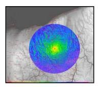
This really looks neat blown up. You can see shadowing behind hills and in river valleys. Uses the Longley-Rice model to predict path loss over irregular terrain.
