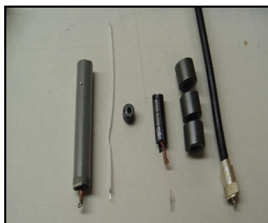
Blown BALUN beside parts used in new BALUN
