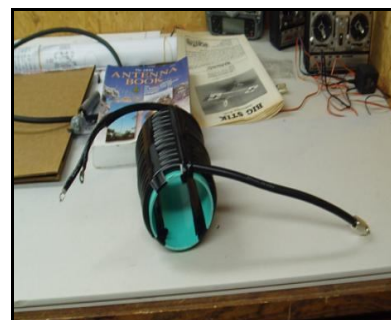
Coaxial BALUN (not used)
