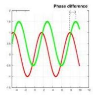
Phase also comes into play in digital circuits where instead of waves, pulses are measured. In a pulse there is rise time, duration and jitter to consider. More on these at another time. Pulses can be out of phase or out of timing with one another just like waves can be out of phase or time with one another.
